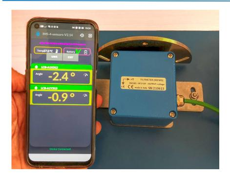
This smart and advanced battery-operated Tiltmeter interface, will turn any standard Tiltmeter with two (4-20mA) wires or 0-5v output to "smart" stand alone device with Bluetooth communication. Free (Android ) Apps allow reading the Tiltmeter from a distance of up to 30 meters (open field) and saving the readings to a history file in excel format. File then can be sent directly from the phone to any email or as a message.
